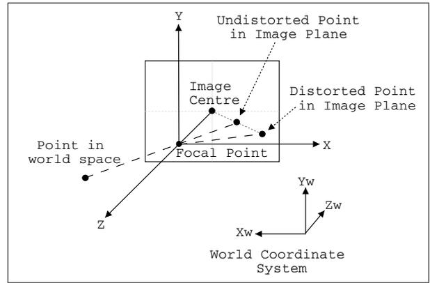
Figure 2: The Pinhole Camera Model
