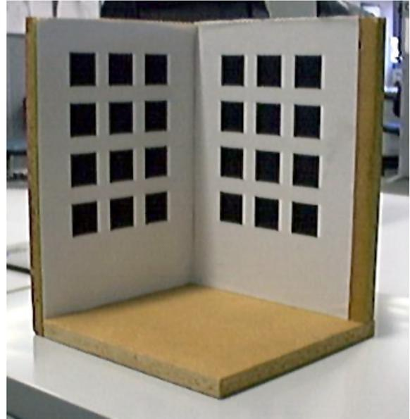
Figure 3: A calibration pattern. The corners of the black squares will be detected and used as calibration points.
