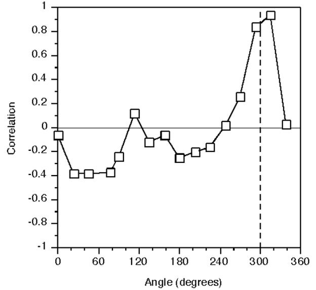
Figure 6 The correlation between a set of reference measurements and readings taken with airflow of 0.35m/s incident at a bearing of 300°.
