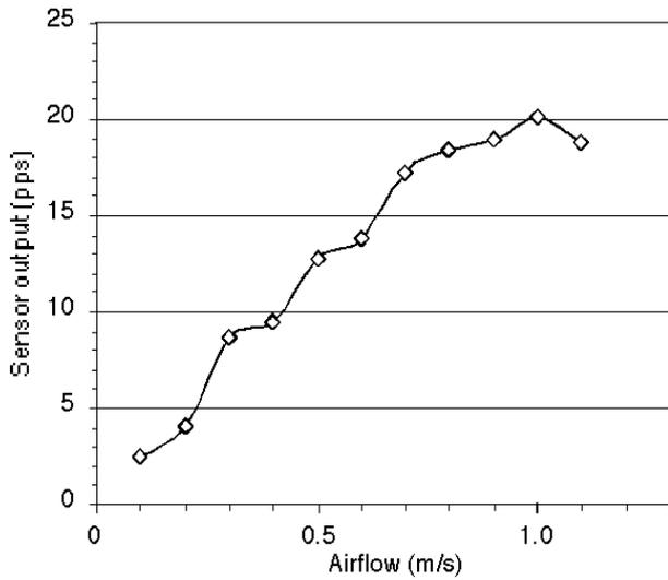
Figure 5 Sensor output positioned at 0 degrees (averaged over 10 seconds) related to airflow velocity.
