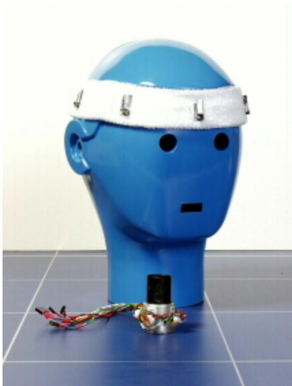
Figure 1 A photograph of the humanoid head with airflow sensing whisker attached to a headband.
