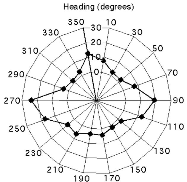
Figure 4 Whisker sensor output in terms of pulses integrated over a 10 second period measured at a wind velocity of  $0.25 \text{ m/s}$ .
