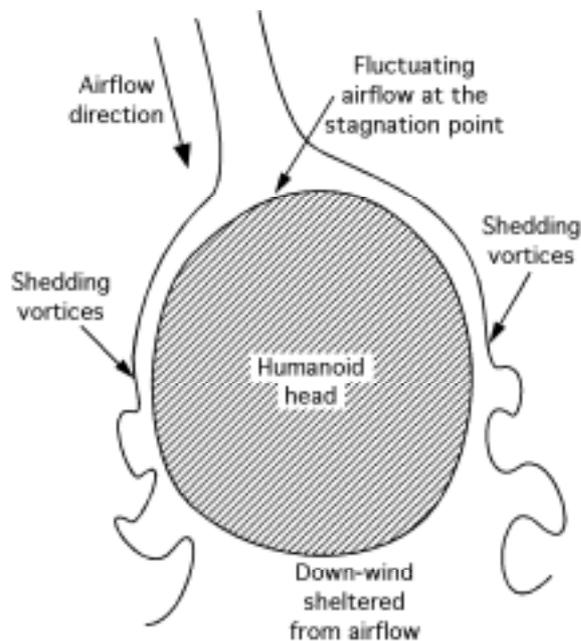
Figure 3 The airflow around the humanoid head.
