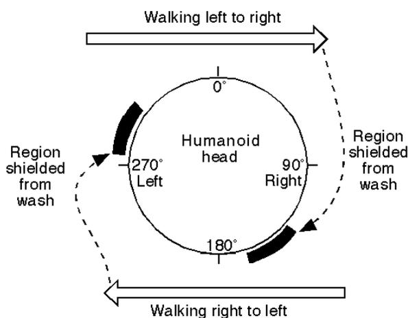
Figure 8 Regions of the humanoid head shielded from the wash of air caused by walking past the head.
