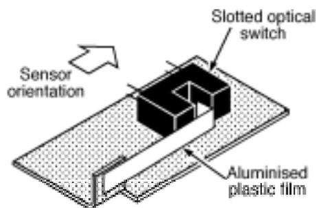
Figure 2 The whisker airflow sensor.
