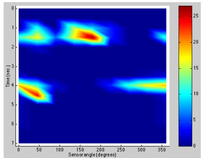
Figure 7 Airflow sensor system response to the wash caused by walking right to left behind the humanoid head and then left to right in front.
