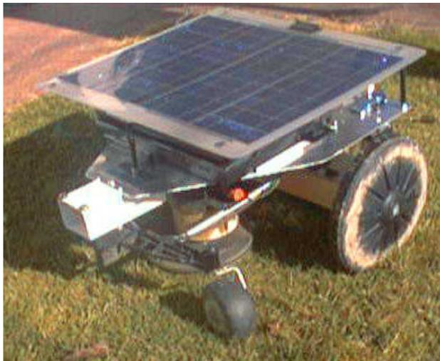
Figure 4: The Robotic Lawnmower in Operation
