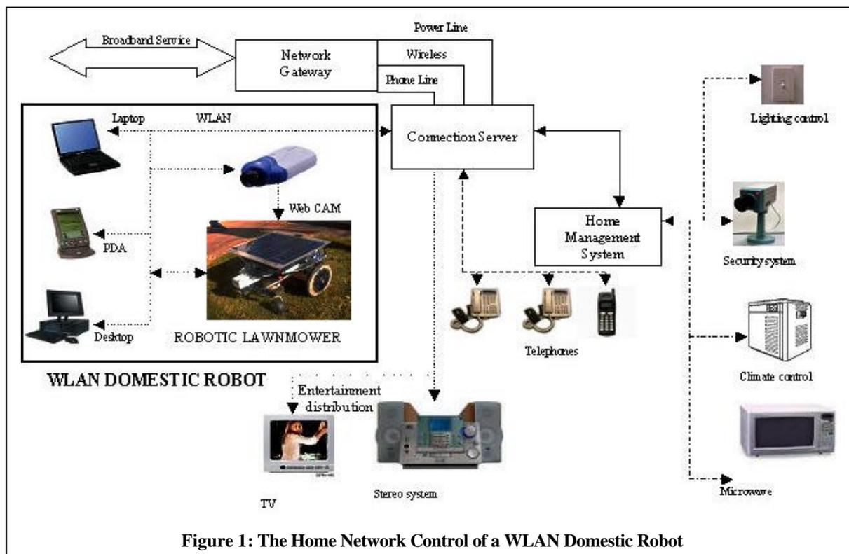
Figure 1: The Home Network Control of a WLAN Domestic Robot
