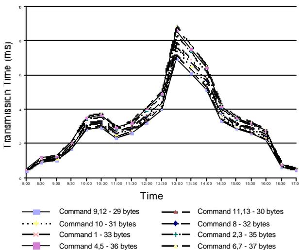
Figure 3: Graph of the transmission times between the Home Controller and the domestic robot.
