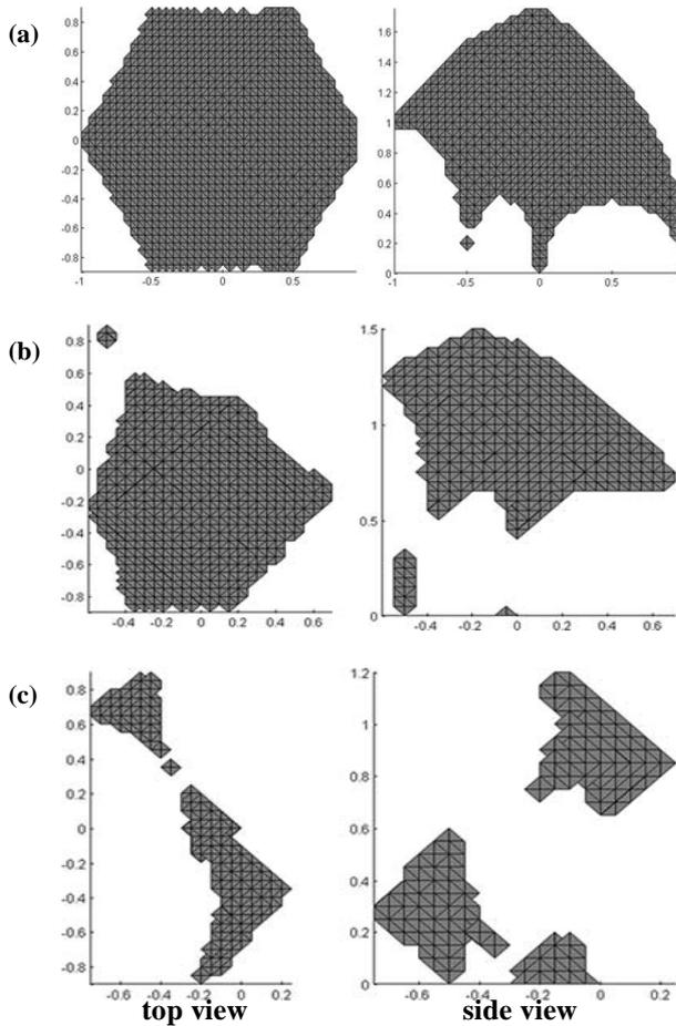
Figure 10 - Constant orientation workspace for MSSM manipulator at (a)  $[0,0,0]$  (b)  $[0,\pi/8,0]$  and (c)  $[0,\pi/4,0]$
