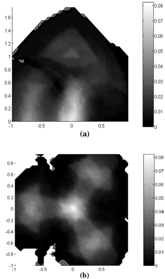
Figure 11 - (a) side and (b) top views of MSSM workspace
