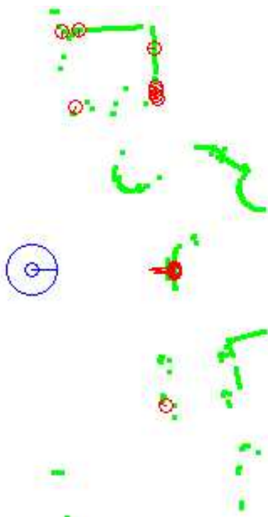
(c) Guesses converge (to the correct location), robot begins to rotate
