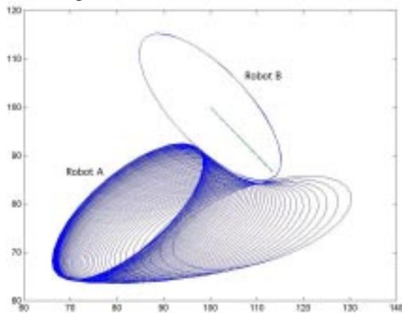
**Fig.8** Simulation result of path behavior of the acoustic navigation model (Robot B is fixed)
