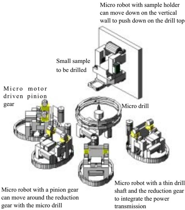
**Fig.1** Overview of microrobots based micro drilling system
