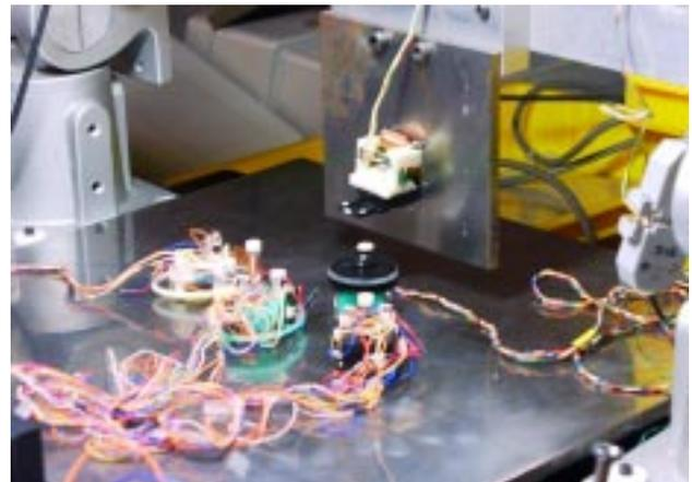
**Fig.10** Experimental setup for automatic micro drilling operation by multiple micro robots.
