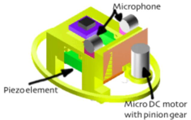
**Fig.3** Miniature robots with a DC motor and microphone
