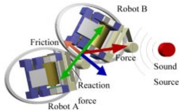
Fig.6 Simple collision model of two small robots with oval outer frame
