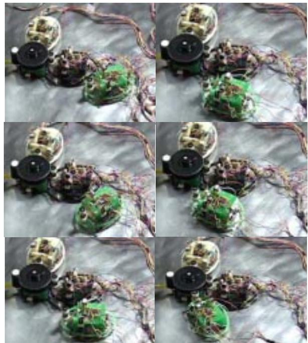
**Fig.9** Three small robots can approach automatically based on the combination of acoustic navigation and oval frame guidance
