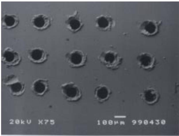
**Fig.12** 15point micro through-hole machined at in the matrix of 0.2mm pitch
