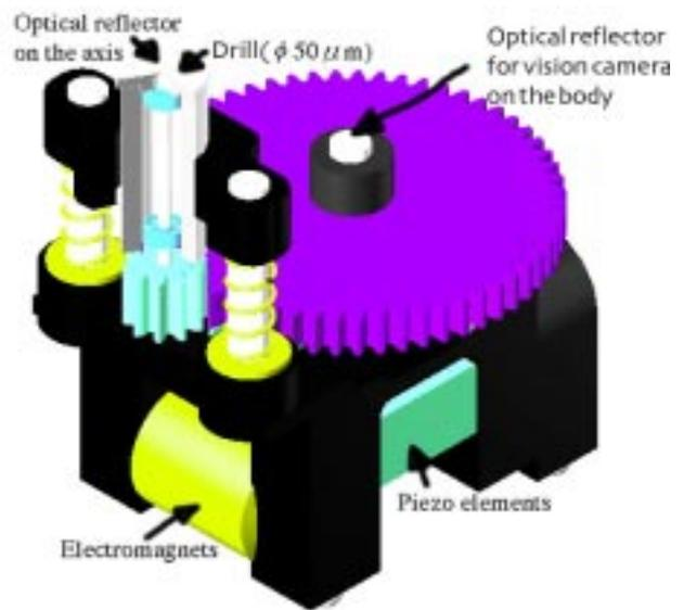
**Fig.2** Miniature robots with micro drill and reduction gear
