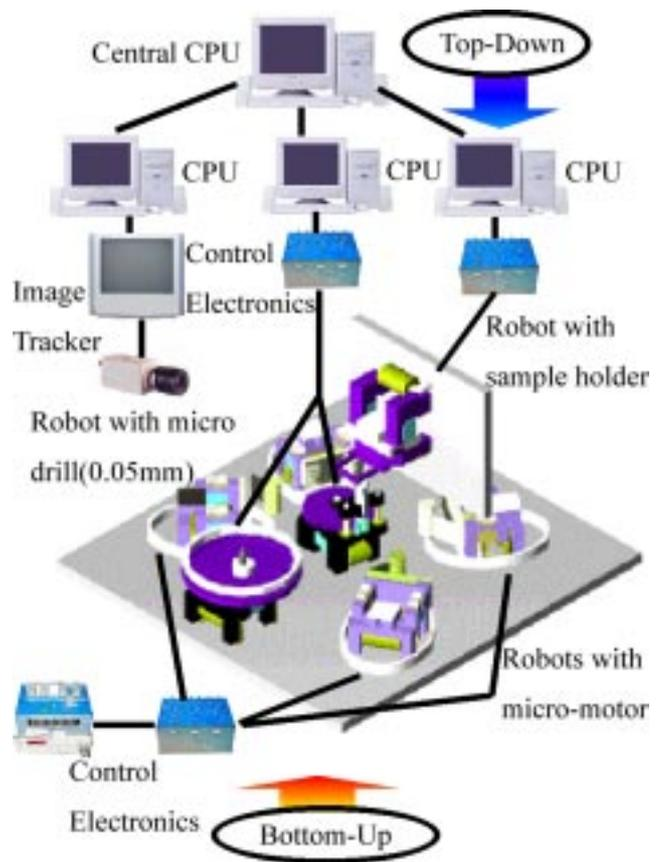
**Fig.5** Control system incorporated with CCD camera vision monitoring system and several PCs.
