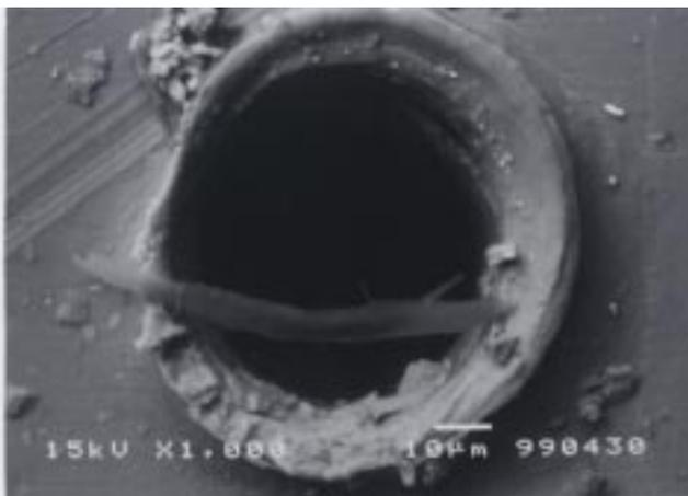
**Fig.13** Micro through hole (0.05mm x 1000 SEM image)
