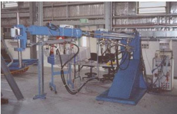
Figure 1: Experimental hydraulic robot arm.
