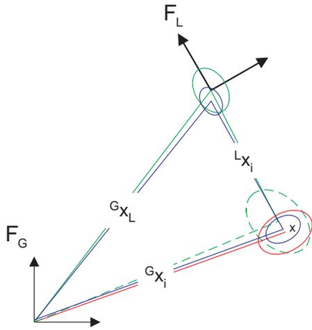
Figure 3: Multiple global feature position estimates in the submap encoding. The light dashed line shows the estimate of feature  $i$  generated through the frame  $\mathcal{F}_L$  while the estimate in the global frame is shown by the solid red line labelled  ${}^G\mathbf{x}_i$ . After constraints are applied, the updated local frame estimate and the estimate of the feature location are also shown.
