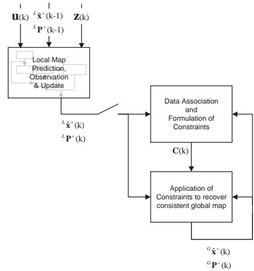
Figure 2: Scheduling of the application of constraints using the Constrained Local Submap Filter. The vehicle operates in a local frame of reference, building an independent map of the features around it. At appropriate intervals, indicated by the switch, the local map is transformed into the global frame of reference and the information fused into the global map using constraints to produce the updated global map estimate.
