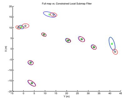
Figure 7: The fused maps of the environment generated by applying consistency constraints to the estimated features. The map is plotted on top of the original map generated by the AMF. There is a very good match between the two maps, as should be expected.
