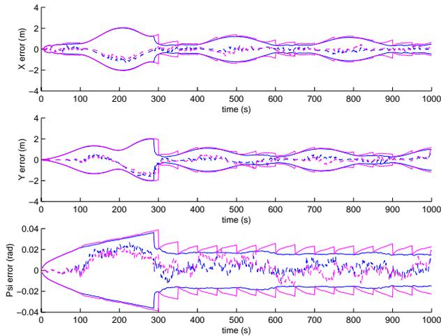
Figure 4: The vehicle estimate errors with the  $2\sigma$  covariance bounds. The AMF SLAM covariance estimates are shown together with the CLSF case. The global vehicle uncertainty grows for the CLSF case between applications of the constraints but the full covariance estimate is recovered when constraints are applied.
