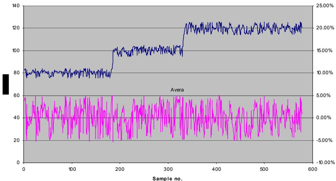
Figure 6: Test results with weight variation (top line) and the percentage variation (bottom line).
