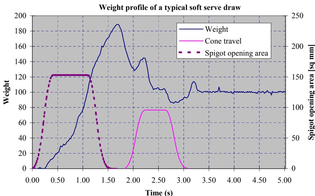
Figure 2:: Typical weight profile with spigot opening and cone travel superimposed.
