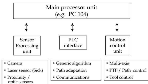
Figure 1: Typical control architecture for variable product processing.
