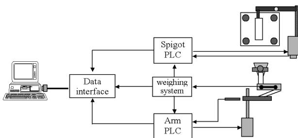
Figure 3: Portion control – laboratory set-up.
