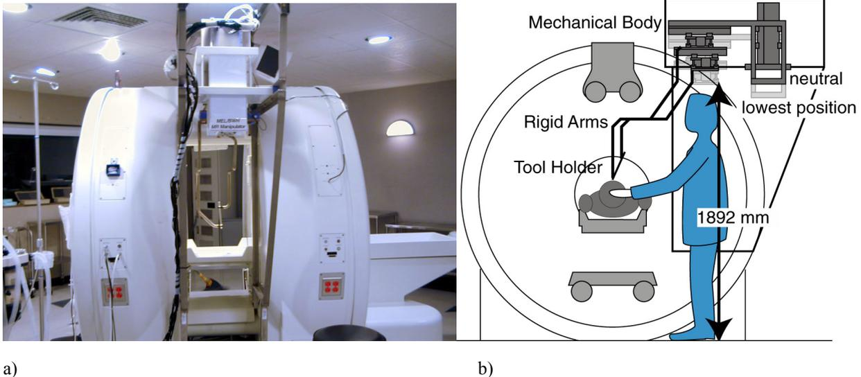
Figure 2. Constructed robot attached to the intra-operative MR scanner (a) and the profile of the workspace (b). The moving part does not obstruct the workspace of the surgeon.
