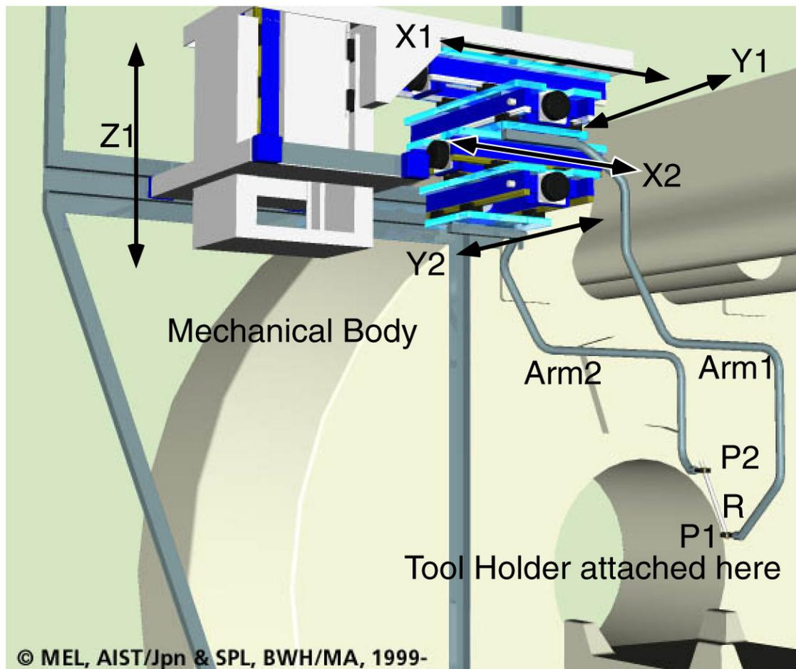
Figure 1. Robot axes layout. X1, Y1, Z1, X2 and Y2 are actuated.
