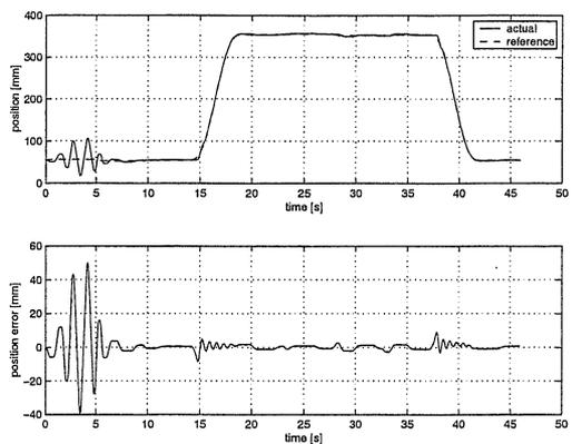
Figure 6: Tracking with MRAC based on a 2nd order model.
