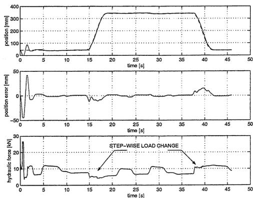
Figure 4: Tracking with varying and changed supply pressure load using MRAC.
