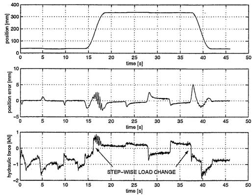
Figure 5: Tracking with varying and changed supply pressure load using VSC.
