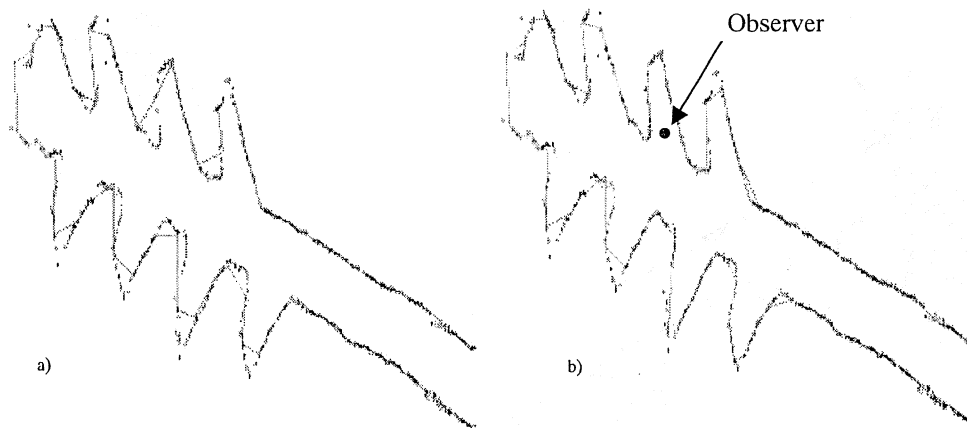
Figure 9. (a) Map with minimum segment length of 3m. (b) Utility run with \alpha=0.33
