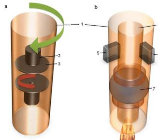
**Fig. 4** Control principles: a) spinning discs for roll, b) gimbale nozzle for pitch and yaw.
