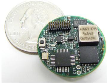
**Fig. 5** The 2g GINA controller board incorporates inertial sensing, processing, communications, and actuation. A MEMS accelerometer and gyros, a 2.4 GHz radio, and a connector to an actuator driver board are visible; the processor is on the backside of the board.
