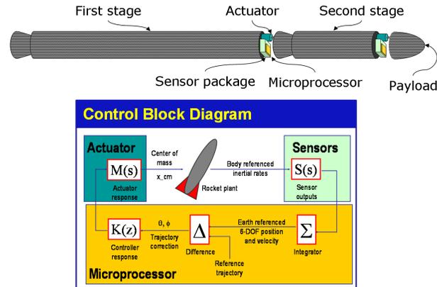
**Fig. 2** A feedback control system can be used to stabilize flight and follow a trajectory. The 6DOF state is sensed by a 6 axis IMU and input to a microprocessor. The current heading and trajectory error is calculated, and a control signal is output to an actuator. The actuator positions a mass or aims the nozzle to induce the appropriate torque on the rocket.
