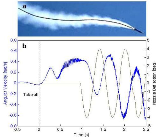
**Fig. 8** a) The sinusoidal smoke trail is generated by thrust vectoring, b) Measured angular velocity demonstrates the rocket's response to pitch control. The oscillation immediately after the take-off is due to unstable flight at low velocities
