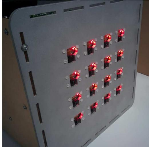
Figure 2: Our Raspberry Pi Camera Array
