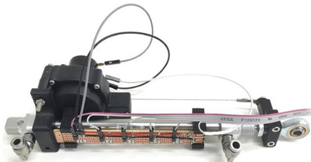
Figure 1: String transducer and Hall Effect sensors array mounted onto a pneumatic cylinder, for gathering data and piston control.
