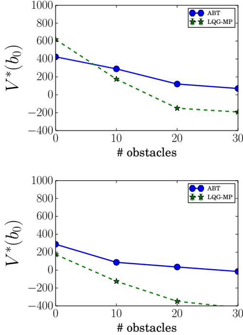
Figure 3: This plot show the mean reward of 50 simulation runs achieved for the car-like robot by ABT and LQG-MP with  $err_{obs} = err_{motion} = 2.5$  (top figure) and  $err_{obs} = err_{motion} = 5.0$  (bottom figure). The  $x$ -axis shows the number of randomly sampled obstacles for each simulation run. The  $y$ -axis shows the mean reward achieved over 50 simulation runs starting from  $b_0$
