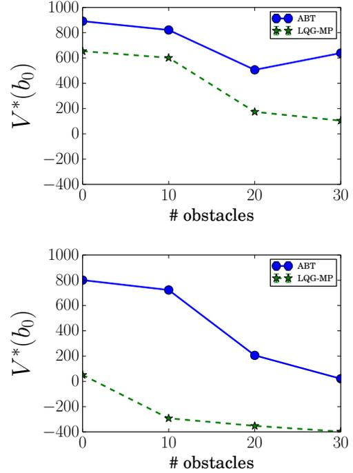
Figure 4: This plot show the mean reward of 50 simulation runs achieved for the manipulator robot by ABT and LQG-MP with  $err_{obs} = err_{motion} = 2.5$  (top figure) and  $err_{obs} = err_{motion} = 5.0$  (bottom figure). The  $x$ -axis shows the number of randomly sampled obstacles for each simulation run. The  $y$ -axis shows the mean reward achieved over 50 simulation runs starting from  $b_0$
