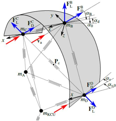
Figure 4: Illustration of the four point mass particle model.  $\alpha$  is the angle of attack,  $v_a$  the apparent air velocity,  $\alpha$  and  $\alpha_0$  depower angles, and  $\alpha_s$  steering angle. Figure adapted from [Fechner *et al.*, 2015].
