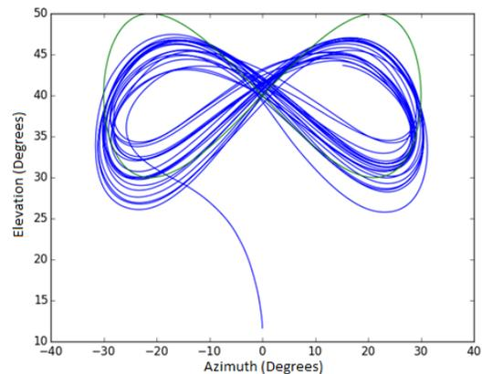
Figure 9: Figure of eight target trajectory, superimposed with flight path of the kite over 4 minutes of simulation. This demonstrates the stability and tracking performance of the controller. The maximum azimuthal range of this trajectory is a little higher than the region where the kite has good traction and therefore could be improved, but the controller succeeds in responding to perturbations and keeping the kite on the target trajectory.
