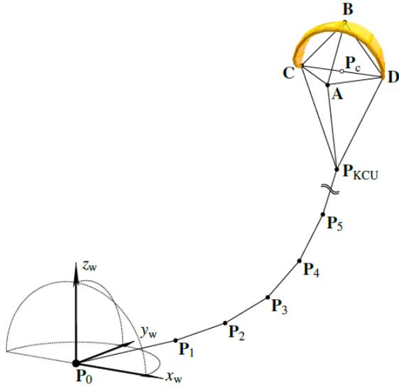
Figure 3: Modelling framework for the tether and kite. The system is made up of discrete point mass particles. Figure adapted from [Fechner *et al.*, 2015]
