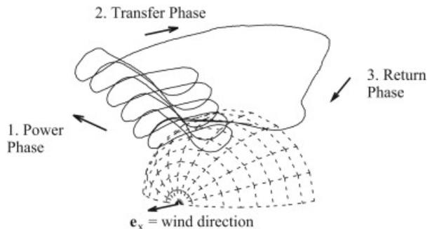
Figure 1: Diagram of the phases of the pumping method of energy generation with a kite power system. The transfer phase is simply the transition from the traction phase to the return phase. Figure adapted from [Erhard and Strauch, 2015].
