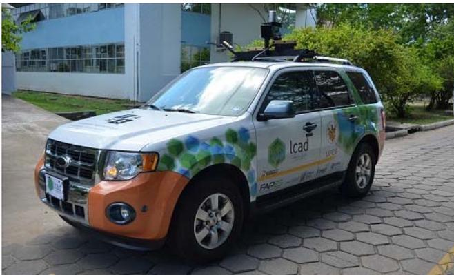
Figure 10: Autonomous platform of the High Performance Computing Lab at Universidade Federal do Espírito Santo, Brazil, named IARA (Intelligent Autonomous Robotic Automobile). This vehicle was used for the experiments in Brazil. The Velodyne sensor is located on the roof of the car.
