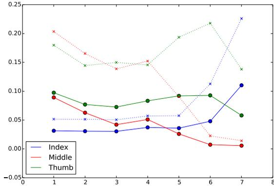
Figure 5: Mean (solid curves) and standard deviations (dashed curves) of all tactile sensors on each finger, at each 1 mm incremental location.
