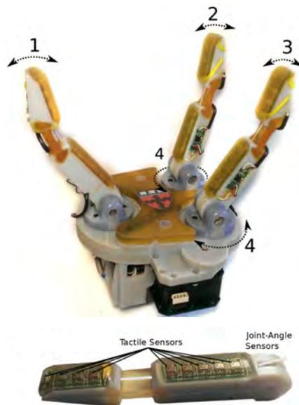
Figure 1: Top: The underactuated hand used here has four actuated degrees of freedom – three for finger flexion, one for coupled rotation of two fingers to transition between wrap grasps and pinch grasps. Bottom: Tactile sensors molded into finger contact surface.
