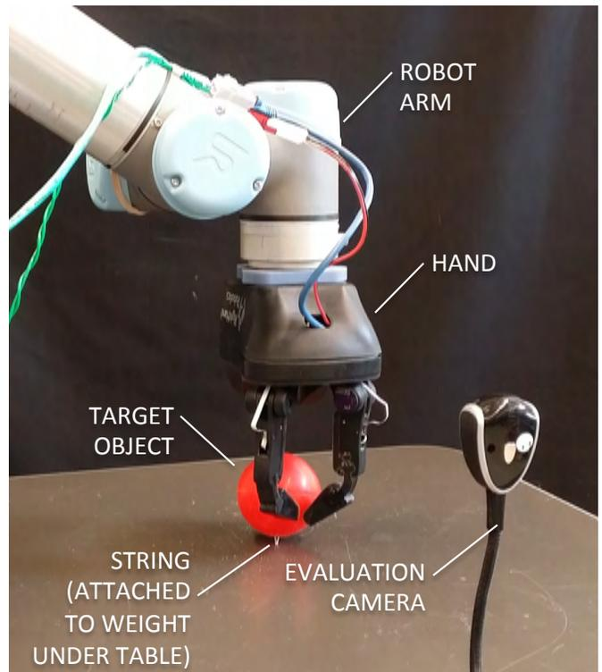
Figure 2: Experimental set up.
