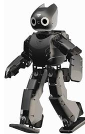
Figure 4: The Robotis DARwIn-OP humanoid robot used as a platform for this research [Ha *et al.*, 2011].
