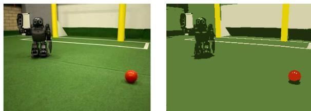
Figure 1: Example of a raw RoboCup image (left) and the equivalent colour-segmented image (right). This segmentation was generated by the unsupervised framework described in [Budden and Mendes, 2013].
