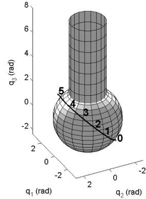
Figure 10: C-space trajectory considering wall obstacle
