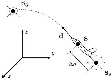
Figure 1: Fluid flow motion planner model
