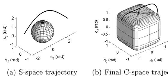
Figure 7: Example of S-space and C-space trajectories
