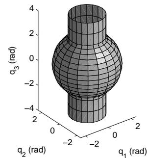
Figure 6: C-space representation of wall obstacle
