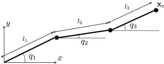
Figure 2: 3-DoF 3R planar manipulator model
