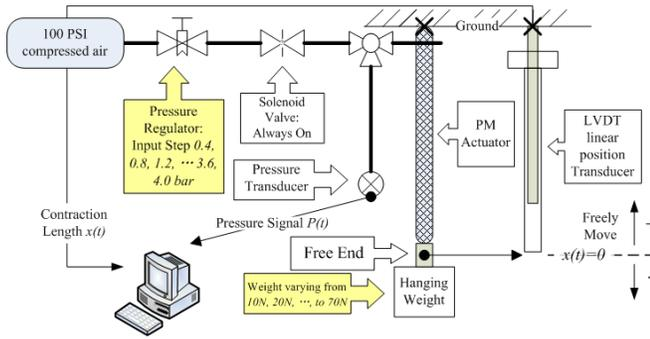
Figure 2. Schematic experimental setup
