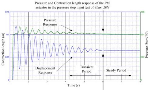
Figure 3. Sample response of the pressure step input experiment (step pressure 4 bar, hanging weight 20 N)
