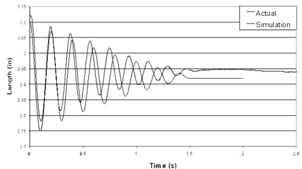
Figure 7: Comparison plot of actuator length vs. time for  $60 \text{ psi}$  nominal pressure and  $6 \text{ lb}$  suspended mass in the test in [Colbrunn et al. 2001]
