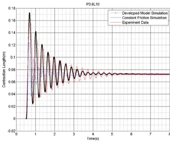
Figure 5: Comparison of results: experimental response (contraction length) with a step pressure input of  $3.6 \text{ bar}$  and load of  $10 \text{ N}$ ; the simulation results from the case with constant Coulomb friction force of  $2.5 \text{ N}$  suggested by [Chou and Hannaford, 1996], and the simulation data obtained by the model (Equation (14))
