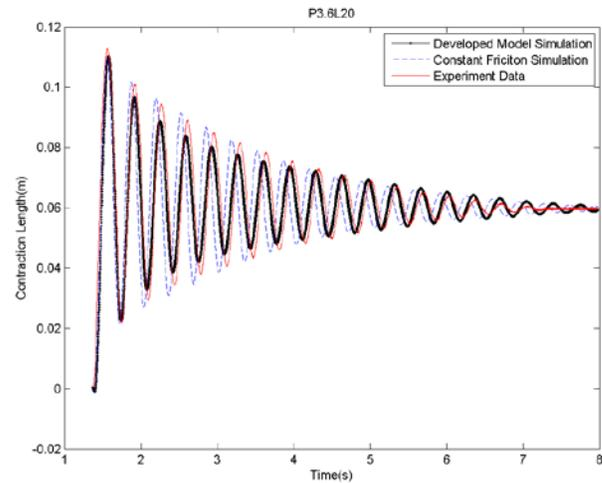
Figure 4: Comparison of results: experimental response (contraction length) with a step pressure input of 3.6 bar and load of 20 N; the simulation results from the case with constant Coulomb friction force of 2.5 N suggested by [Chou and Hannaford, 1996], and the simulation data obtained by the model (Equation (14))
