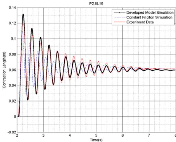
(a) Simulation and experimental results of the case of  $(2.8 \text{ bar}, 10 \text{ N})$
