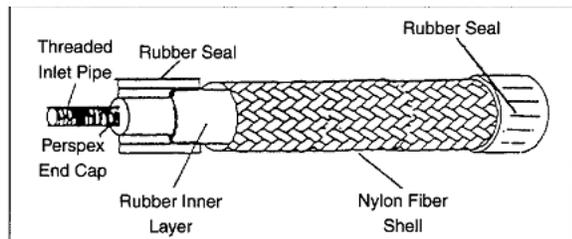
Figure 1: Structure of the pneumatic muscle ([Caldwell et al. 1995])
