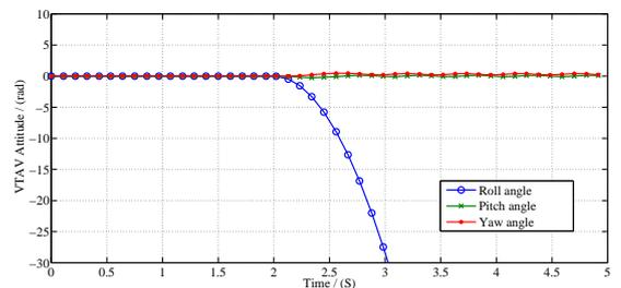
Figure 13: Attitude response of nonlinear model under impulse disturbance
