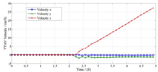
Figure 12: Velocity response of nonlinear model under impulse disturbance
