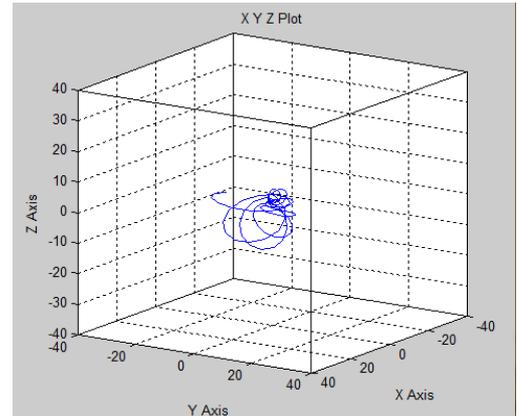
Figure 11: Translation of linear model under impulse disturbance
