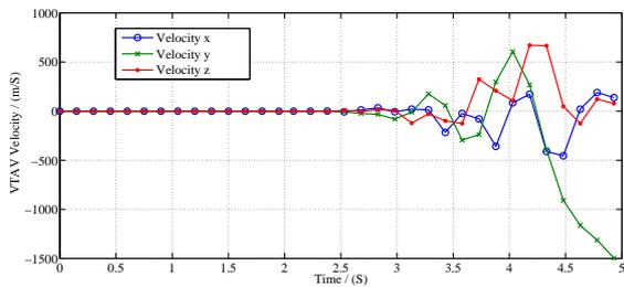
Figure 9: Velocity response of linear model under impulse disturbance
