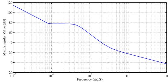
Figure 4: Frequency response of Maximum Singular Value of the System
