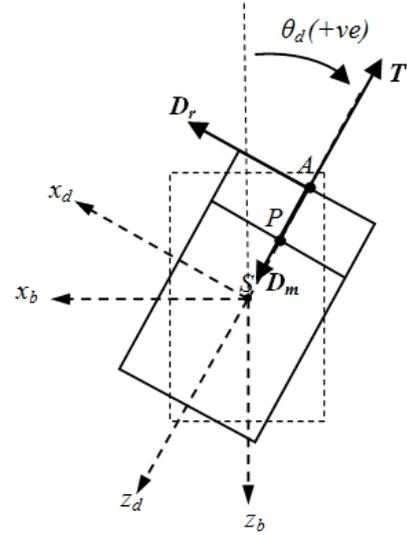
Figure 3: Forces acting on a single duct. T-Thrust
