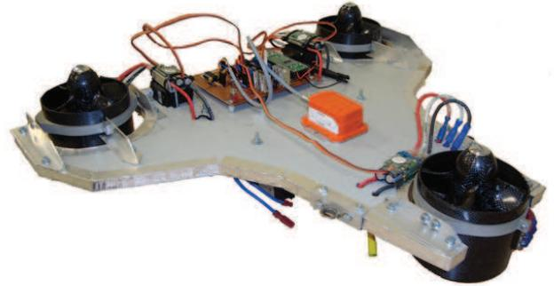
Figure 1: Vectored Thrust Aerial Vehicle (VTAV)
