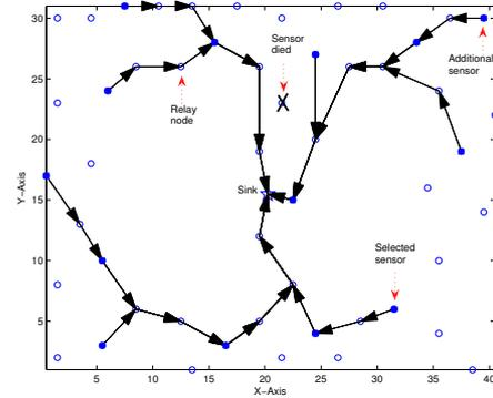
Figure 3: Sensors chosen and deployed in Intel Berkeley Lab when one sensor died, and optimal routing structure on the network: Square indicates the locations selected; circle indicates the locations unselected;  $\times$ -mark shows the sensor died
