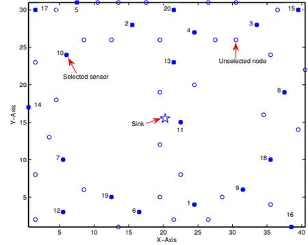
Figure 1: 20 out of 52 sensors chosen by simulated annealing based algorithm and ordered through information, deployed in Intel Berkeley Lab: Square indicates the locations selected; circle indicated the locations unselected
