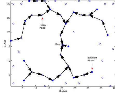
Figure 2: Sensors chosen and deployed in Intel Berkeley Lab with all sensor nodes, and optimal routing structure on the network: Square indicates the locations selected; circle indicates the locations unselected
