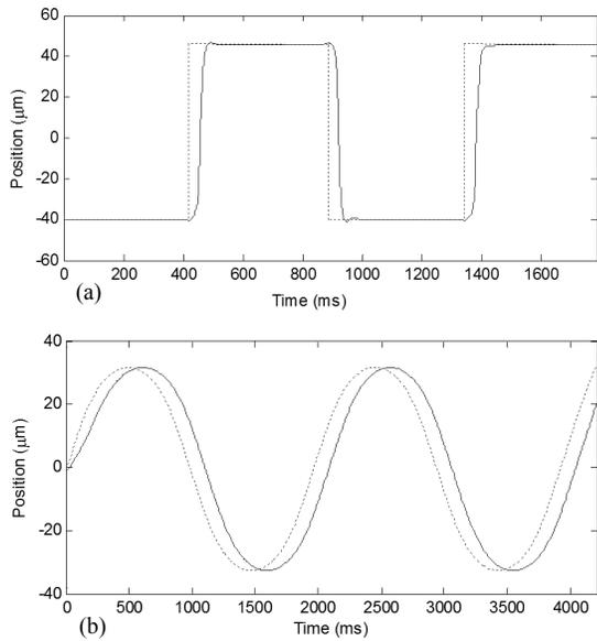
Figure 8. Control system response to the desired trajectory. (a) square wave response in coarse mode (b) Sinusoidal wave response. Dashed red line and solid blue line indicate desired trajectory and control system actual responses respectively.
