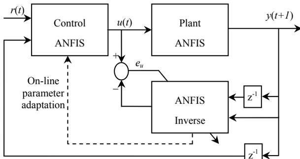
Figure 7. Block diagram of adaptive learning. On-line learning of ANFIS inverse model occurs at each time step to fine-tune the membership function parameters of ANFIS controller.
