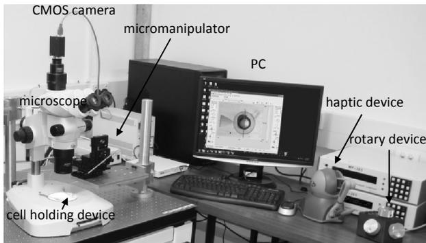
Figure 2. Haptic microrobotic cell injection system.
