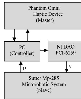
Figure 3. Control system architecture.  $v$  is the voltage level and  $p$  is the position feedback.
