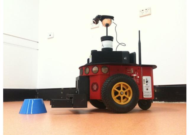
Figure 1: The Pioneer robot used for experiments. The camera was placed to give as large a field of view as possible while still viewing the contents of the gripper. The object used was a distinct blue plastic marker.
