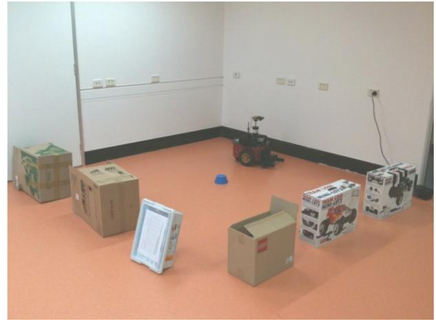
Figure 4: The arena for study 3. A 2.5m x 2.5m area was cordoned off by large obstacles that could be detected by the laser range finder. The Pioneer was set to roam inside the area while avoiding the blue object.
