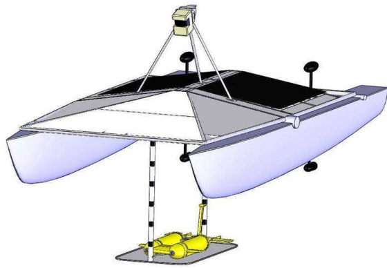
Figure 2: Conceptual diagram of AUV docking system slung underneath the CSIRO developed Nikki Autonomous Surface Vehicle.
