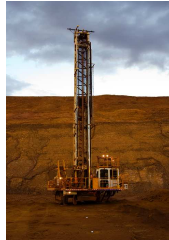
Figure 1: An autonomous blast hole drill rig used for collecting experimental MWD data in this paper.
