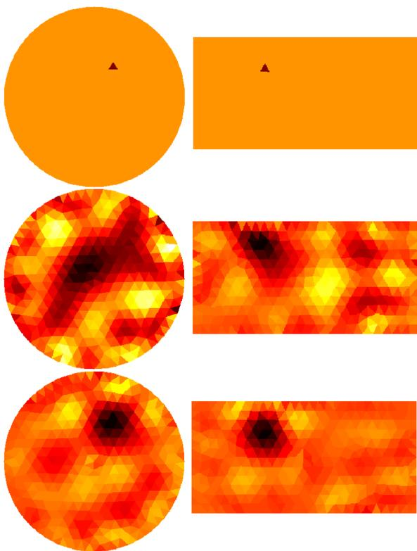
Figure 9: Reconstruction for different drive patterns with  $7\mu\text{V}$  RMS noise. Stimulus (top), adjacent drive pattern (middle), adjacent injection pattern and centre measurement pattern (bottom).
