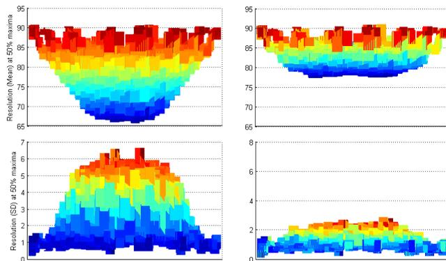
Figure 8: Lateral view of resolution at 50% maxima in a circular geometry and  $7\mu\text{V}$  RMS noise. Adjacent (left column) and centre (right column) measurement patterns. Mean (top row) and standard deviation (bottom row) of all element in the mesh.
