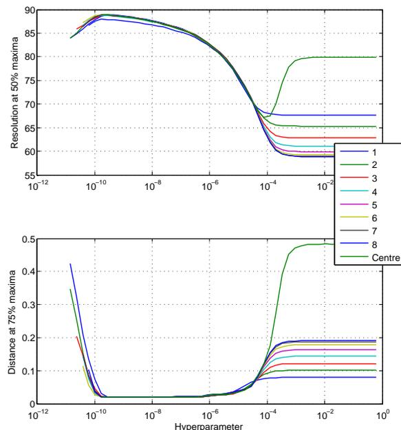
Figure 4: Resolution (top) and distance error (bottom) curves for a circular geometry, centre measurement pattern and nine current injection patterns.
