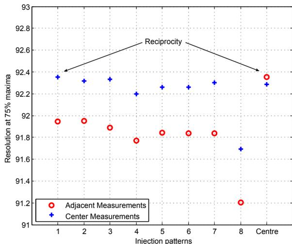
Figure 7: Resolution at 75% maxima for a circular geometry, adjacent and centre measurement patterns and nine current injection patterns.
