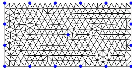
Figure 3: Finite element discretisation for a rectangular body with 17 electrodes, shown in blue.
