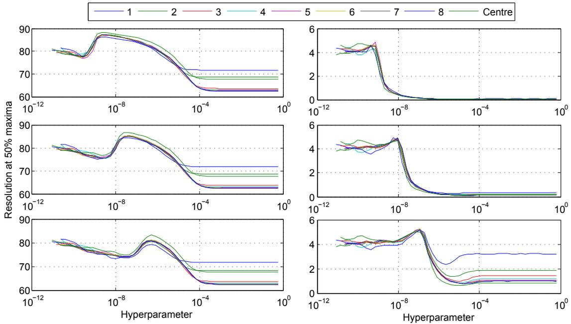
Figure 5: Resolution at 50% maxima. Mean (left) and standard deviation (right) curves for a circular geometry, adjacent measurement pattern and 9 current injection patterns with fixed Gaussian noise levels increasing from top ( $.07\mu\text{V RMS}$ ) to bottom ( $7\mu\text{V RMS}$ ). A total of 200 reconstructions were performed for each element.
