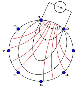
Figure 1: Likely equipotential lines (in red) for a circular 2D body with current injected through a pair of adjacent electrodes.
