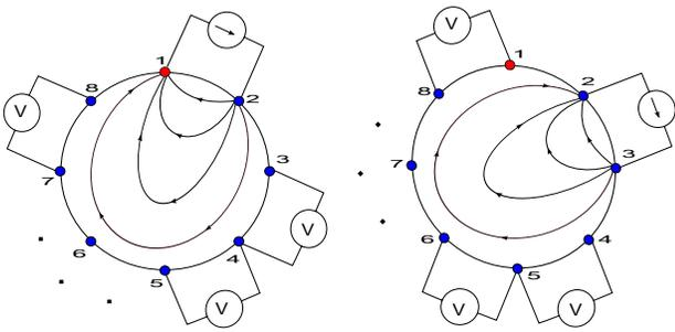
Figure 2: First (left) and second (right) steps for the adjacent drive pattern.
