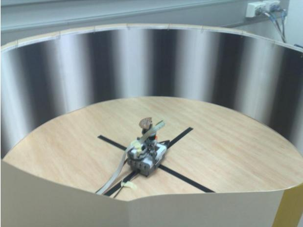
Figure 10 – The testing arena for the one-dimensional sensor array. The sinusoidal grating provides an exemplary environment for assessing the egomotion measurement characteristics of the sensor.
