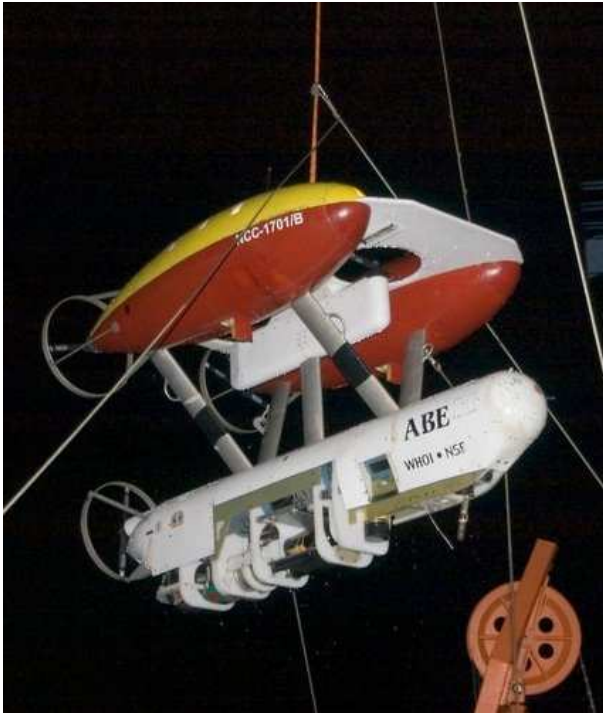
Figure 1: The ABE AUV being deployed on a hydrothermal vent prospecting mission in 2005 on the Southern Mid-Atlantic Ridge near Ascension Island. Various acoustic sensors in the lower pod measure vehicle velocity over ground and through water, collect soundings of sea floor depth, and collect rangings to fixed acoustic beacons. Hydrographic sensors located near the nose of the starboard and lower pods collect physical oceanographic data and record the concentration of various hydrothermal tracers.
