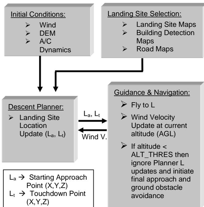
Figure 1 - Emergency Landing Software System
