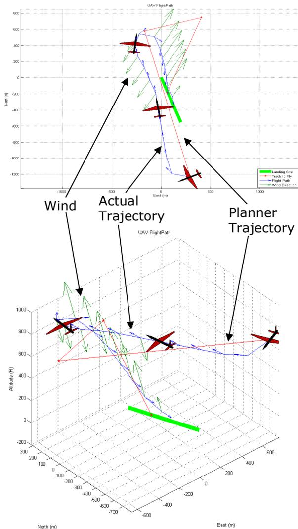
**Figure 6 – Detailed View of the Forced Landing Simulations under Changing Wind. Green arrows indicate the direction of the wind.**
