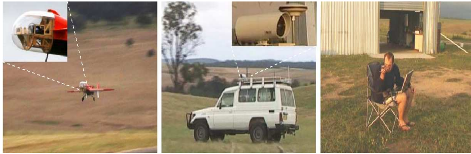
Figure 4: Data is obtained from multiple sources including cameras mounted on an autonomous air vehicle and ground vehicle. Observations are also submitted to the system by human operators. Each of the different sensor modalities are incorporated into our filtering scheme. Close-ups of the sensor payloads including monocular colour cameras are shown in the insets.
