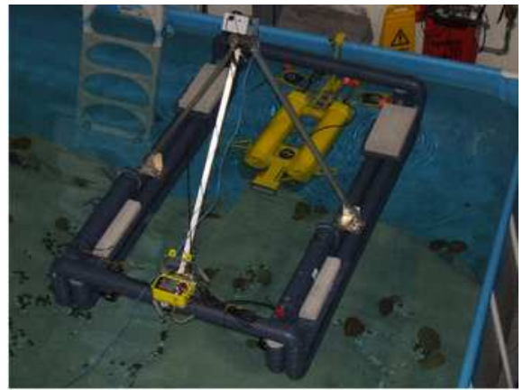
Figure 11: The Starship ASV after docking with the AUV during a pool experiment.
