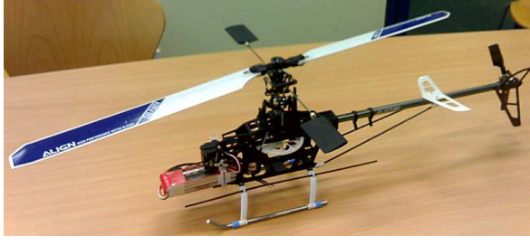
Figure 4: A model helicopter platform built for flying experiments.
