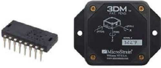
Figure 3: Agilent optical-mouse chip (left) and MicroS-train 3DMG inertial measurement unit (right) used for experiment.
