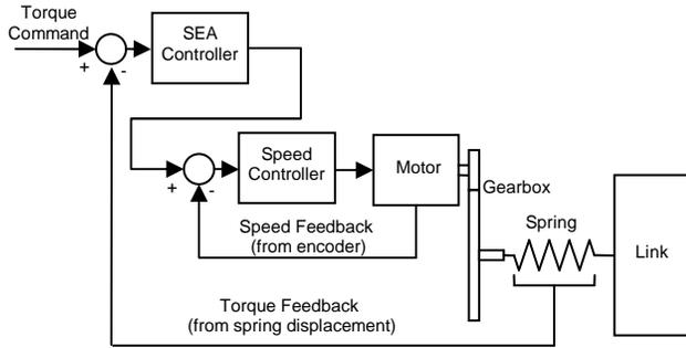
Figure 1: The inner velocity loop in the velocity sourced SEA helps to overcome problems with non-linearities and stiction
