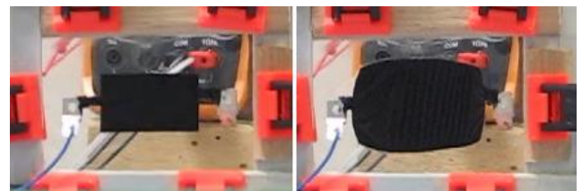
Figure 3: VHB 4910 with 200,200% prestrain in initial and actuated states.
