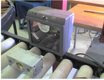
Fig.5. The PSC VS1200 barcode reader used for part identification
