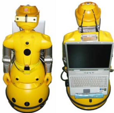
Figure 1: Wakamaru with Bumblebee camera on head, HokuyoURG laser range finder at middle and laptop on back.
