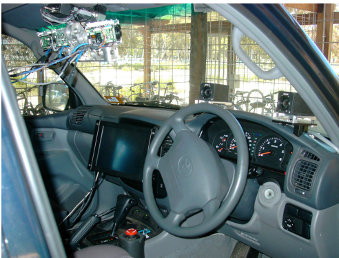
Figure 1: Inside the ANU/NICTA intelligent vehicle. Cameras to monitor the road scene appear in place of the rear-vision mirror.
