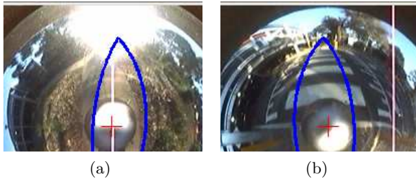
Figure 9: Two instances of tracking failures. (a) Frame 754, caused by sun glare obscuring the road ahead. (b) Frame 2487, caused by the pedestrian crossing not having a significantly different colour distribution from its surroundings.
