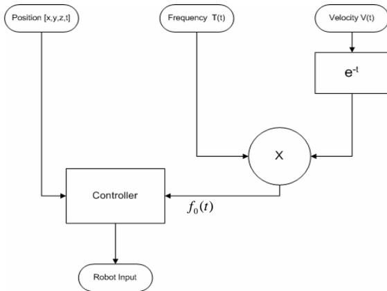
Figure 9. Haptic to robot controller
