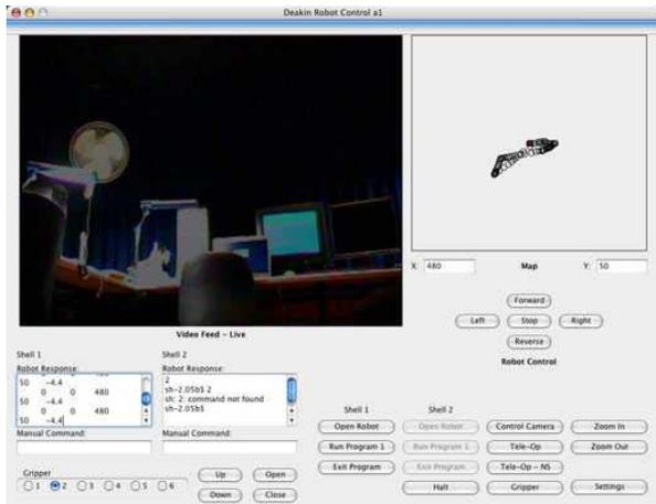
Figure 2. Haptic server software configured for ActivMedia P3-AT robot.
