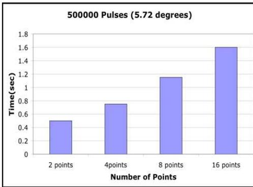
Figure 6. Epson Join 1 movement with respect to time (small rotation)
