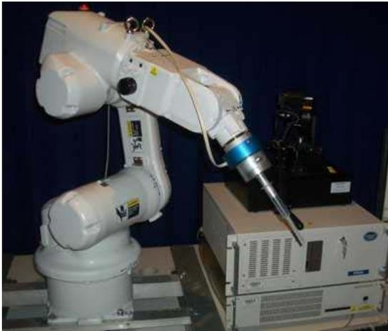
Figure 3. Epson Pro Six fitted with JR3 force/torque sensor ready for a haptically controlled needle insertion task.
