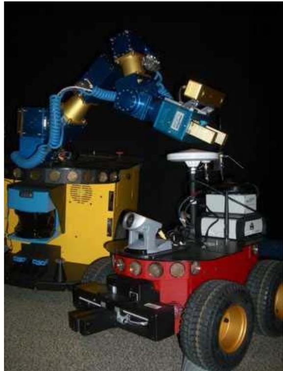
Figure 4. ActivMedia Powerbot and P3-AT series robot's configured for haptic control. Note the PowerCube arm on the larger Powerbot.
