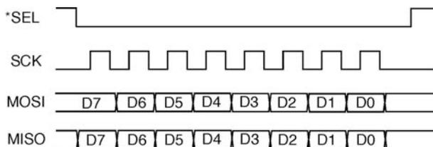
Figure 6 SPI interface protocol.
