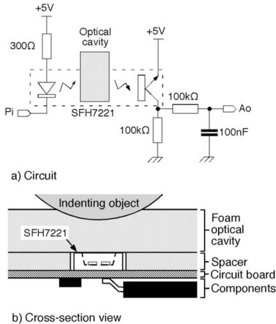
Figure 1 One touch-sensitive element in the sensor array.
