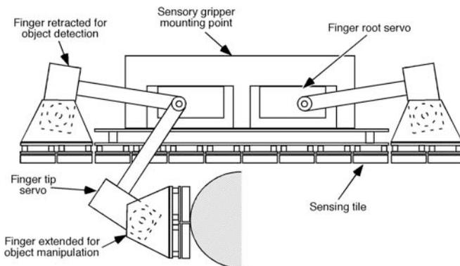
Figure 9 A side view of the sensory gripper.
