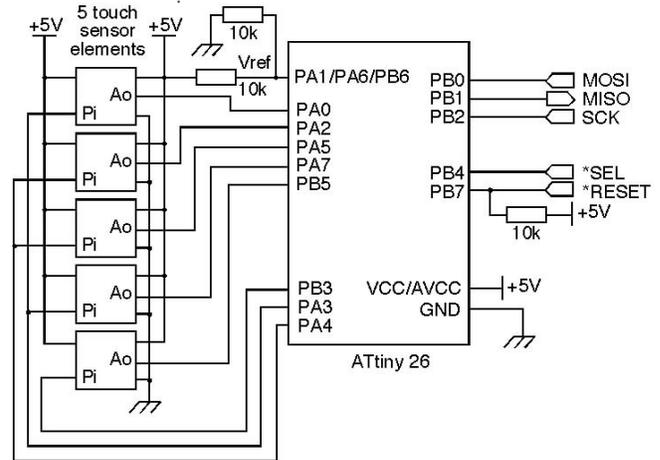
Figure 3 The circuit contained in one sensor tile.
