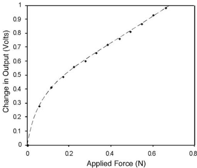
Figure 2 The relationship between applied force and change in output voltage for one taxel of the sensor array.
