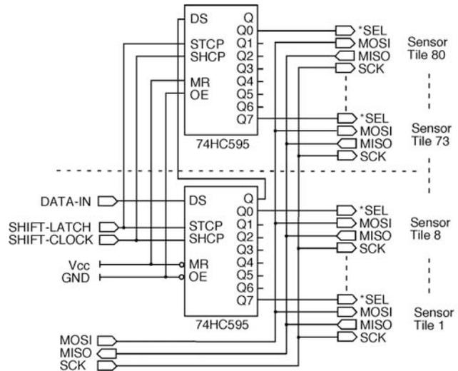
Figure 7 Sensor tile select circuitry.
