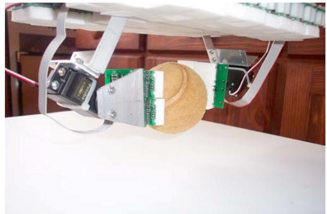
Figure 10 The sensory gripper grasping a tennis ball
