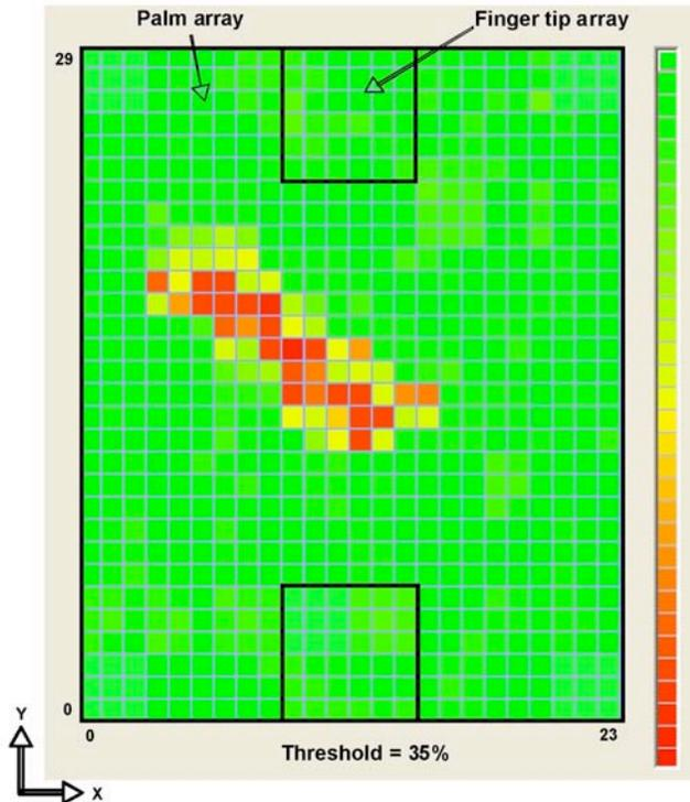
Figure 8 A tactile image produced by the tactile sensor array.
