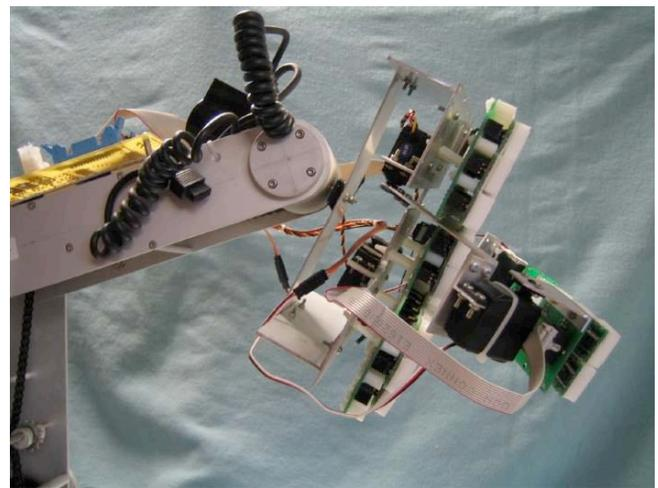
Figure 11 The sensory gripper and SIR 1 robot manipulator.
