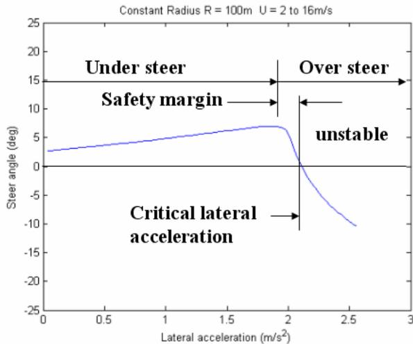
**Figure 7: Predictions of steering angle ( $\delta$ ) required on the tractor, for a constant radius (100m) turn,  $2 < U < 16$  m/s.**
