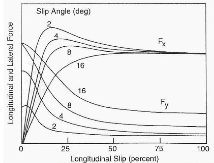
Figure 4: Typical tyre characteristics during braking.
