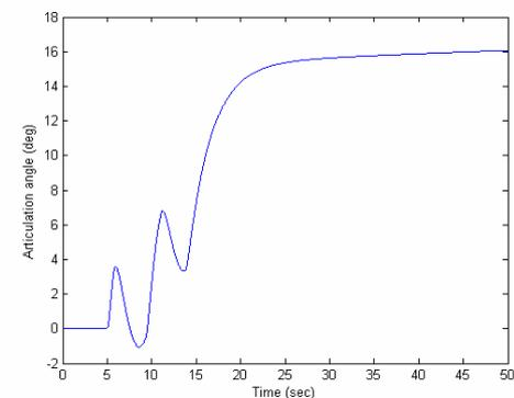
**Figures 12: Transient responses for step steering input of  $\delta=20$  degrees applied after five seconds with forward velocity 15 m/s.**
