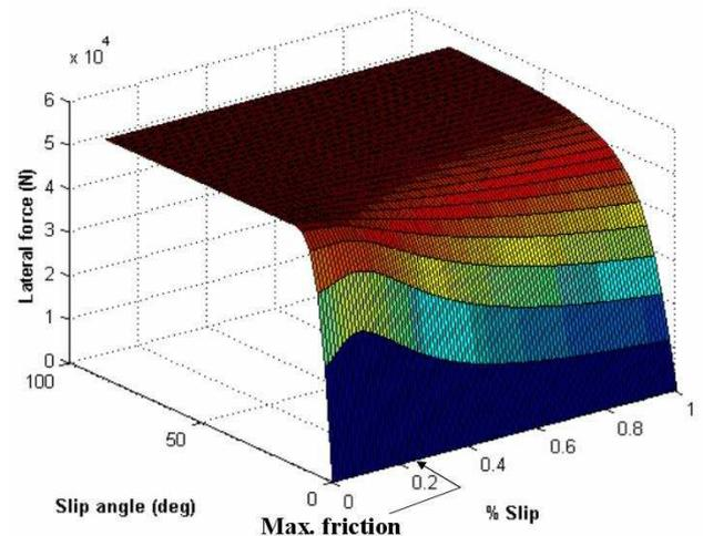
Figure 5: Modelled tyre characteristics Caterpillar 776D tractor and trailer during braking.
