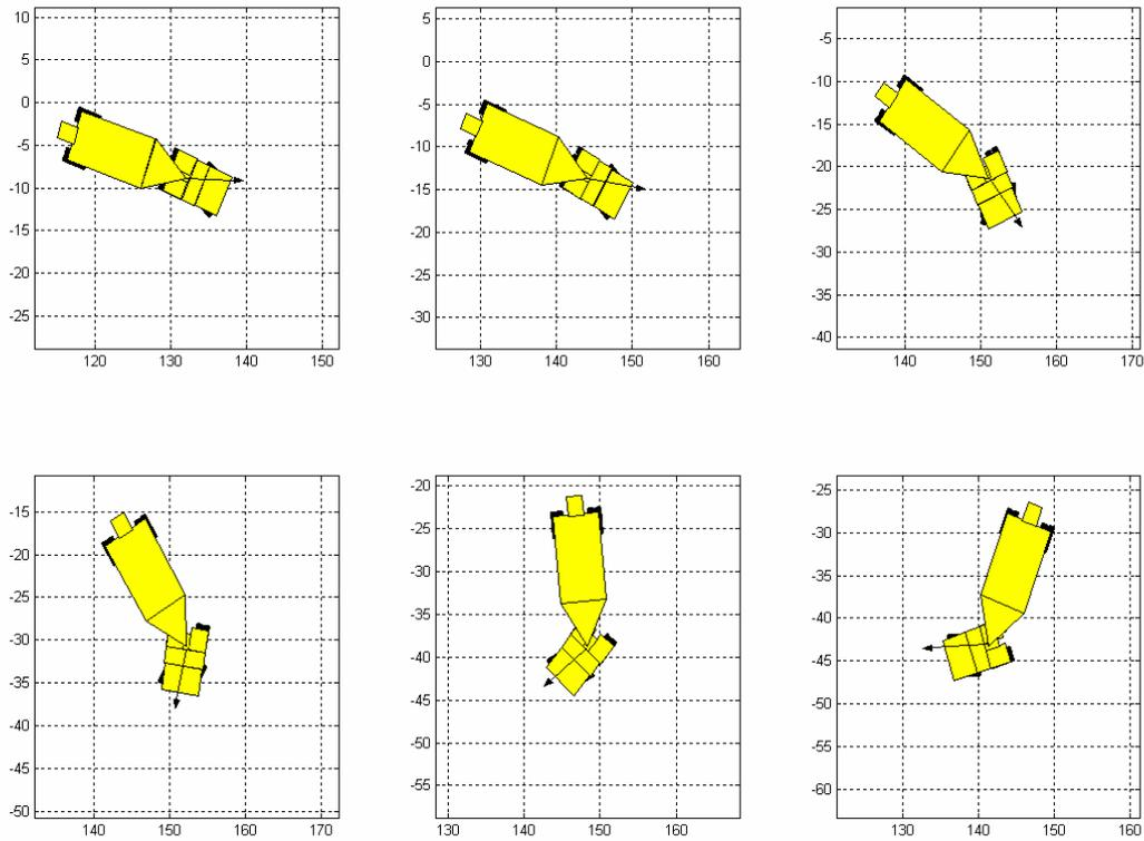
**Figure 13:** Responses for step steering input of  $\delta=20$  degrees applied after five seconds with forward velocity 15 m/s. Vectors show the direction of the velocity vector.
