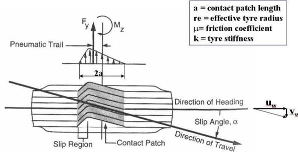
Figure 3: Tyre parameters and state variables.
