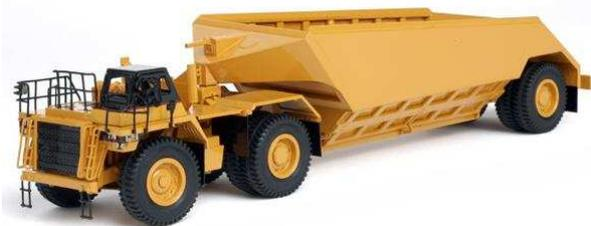
Figure 1: Caterpillar 776D tractor and trailer. Engine power 700KW, 56 tonnes (empty), load 160 tonnes.
