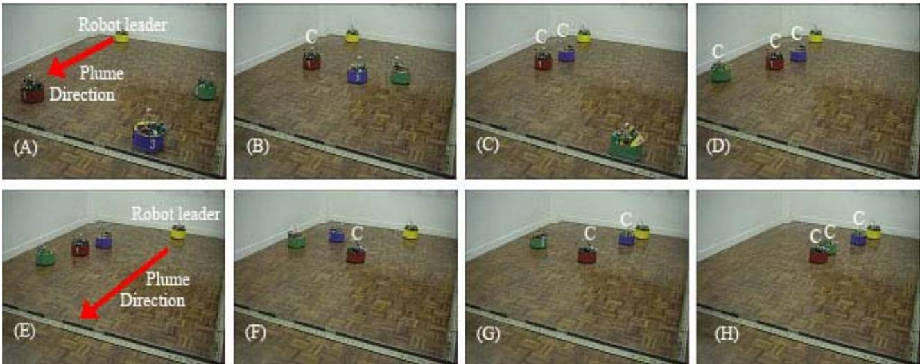
Figure 10. Congregation behaviour using a robot leader and other three robots (C indicates a robot that has congregated in the plume).
