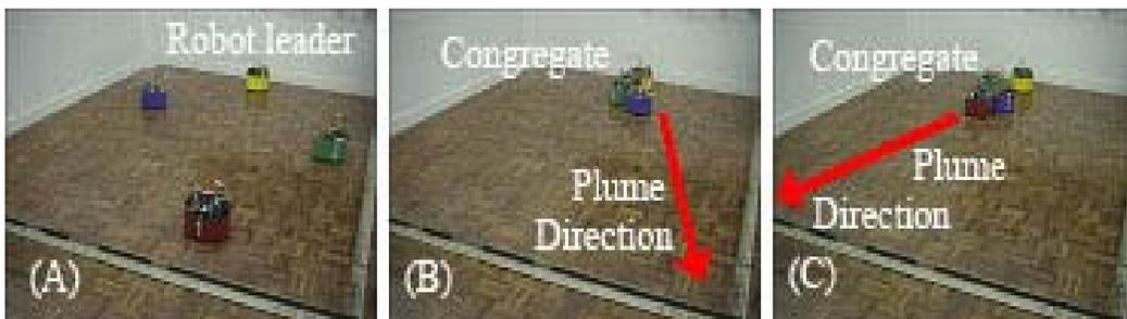
Figure 11. Congregation behaviour resulting from projecting the plume in different directions.
