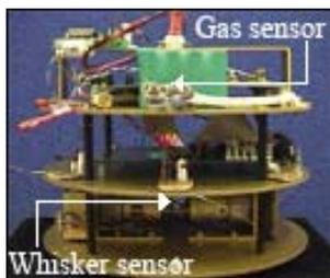
Figure 1. A mobile robot equipped with an odour sensor and three whisker sensors.
