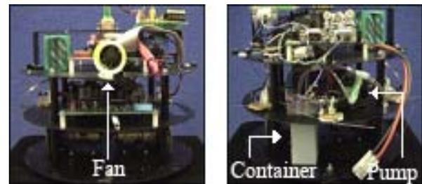
Figure 2. The robot leader carrying a pump, chemical container and fan.
