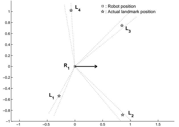
Figure 1: The cones rooted at the first observation point  $R_1$  contain the landmarks. Each cone represents the uncertainty of the bearing of the associated landmark. The diagram is drawn with respect to the robot frame  $\mathcal{F}_R$ .
