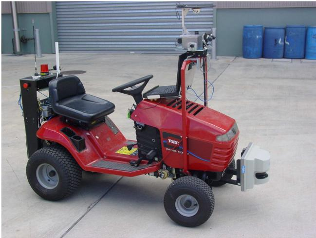
Figure 3: Ground vehicle platform : Automated ride-on lawn mower fitted with GPS, IMU, laser rangefinder and a number of Firewire cameras. The vision processing and control computers are fitted behind the driver's seat.
