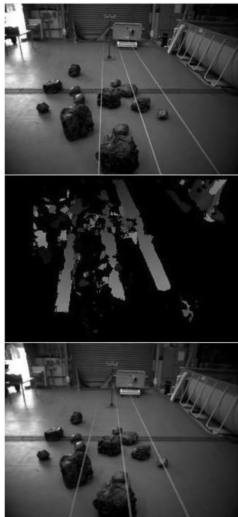
Figure 8: Tertiary image taken from aerial pod of scale-model power lines. The disparity between the right (top) and left (bottom) image is used to create a range image (middle).
