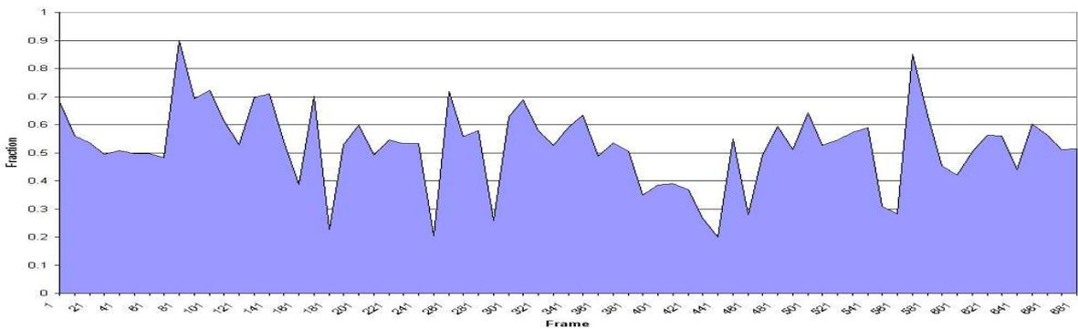
Figure 10: Fraction of matches fitting expected epipolar geometry from calculated fundamental matrix
