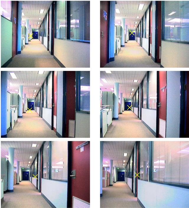
Figure 11: Frames from robot camera sequence showing epipole
