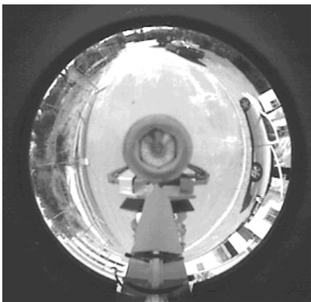
Figure 1: Robot's view of its environment through an omnidirectional camera, the sensor that RatSLAM uses to maintain its localisation. The robot is facing towards the top of the image. The support for the mirror obscures part of the robot's field of the view towards its rear.
