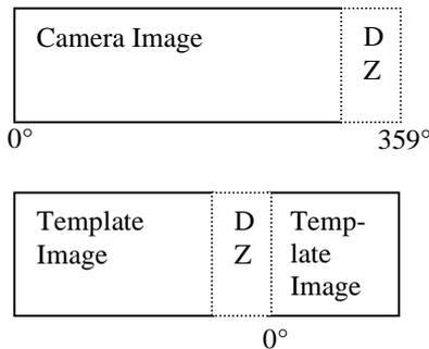
Figure 3: When rotating the template image to determine at what orientation it best matches the current camera image the camera's dead zone must be taken into account. The robot has no knowledge of what lies in the dead zone in either the current or template images so these areas cannot be compared.
