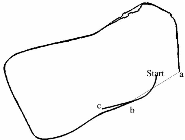
Figure 8: RatSLAM trajectory while completing two forward traversals of the route shown in Figure 6. During the second lap the RatSLAM recognizes that it is repeating a learnt path and adjusts its perceived position from *a* to *b*. Re-localisations are shown as thin lines.
