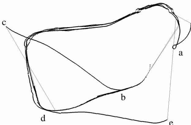
Figure 10: RatSLAM trajectory while completing three forward and one backwards traversals of the route shown in Figure 6. The robot performs a  $180^\circ$  turn at the point *a* and maintains a consistent path up to point *d*, despite travelling in the opposite direction to the one it has experienced. On the third and fourth circuits the robot is unable to maintain its localisation all of the time resulting in the incorrect path sections *b-c* and *d-e*.
