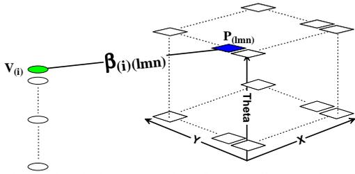
Figure 4: The local view network and pose cell network. Activated units in the local view,  $V_i$ , become associated with activated units in the pose cells,  $P$ , through learnt weighted connections between the two networks. The relative orientation of the robot reported by the vision system is used to dynamically change the Pose Cells each LV-PC link is connected to.
