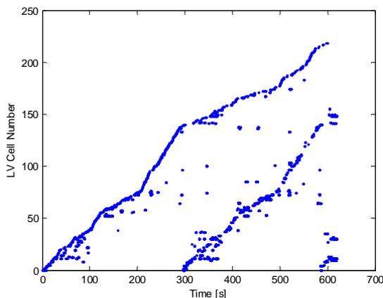
Figure 7: Activated Local View (LV) units versus time as the robot traverses the environment. For any given input zero or more templates may be found. Beginning at 300 seconds the robot begins to retrace its path and re-encounter previously seen views, resulting in repeated patterns of Local View activity.
