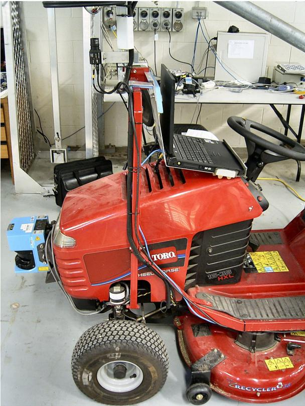
Figure 5: The autonomous tractor. The omnidirectional camera and mirror assembly is mounted on an elevated point above the front wheels.
