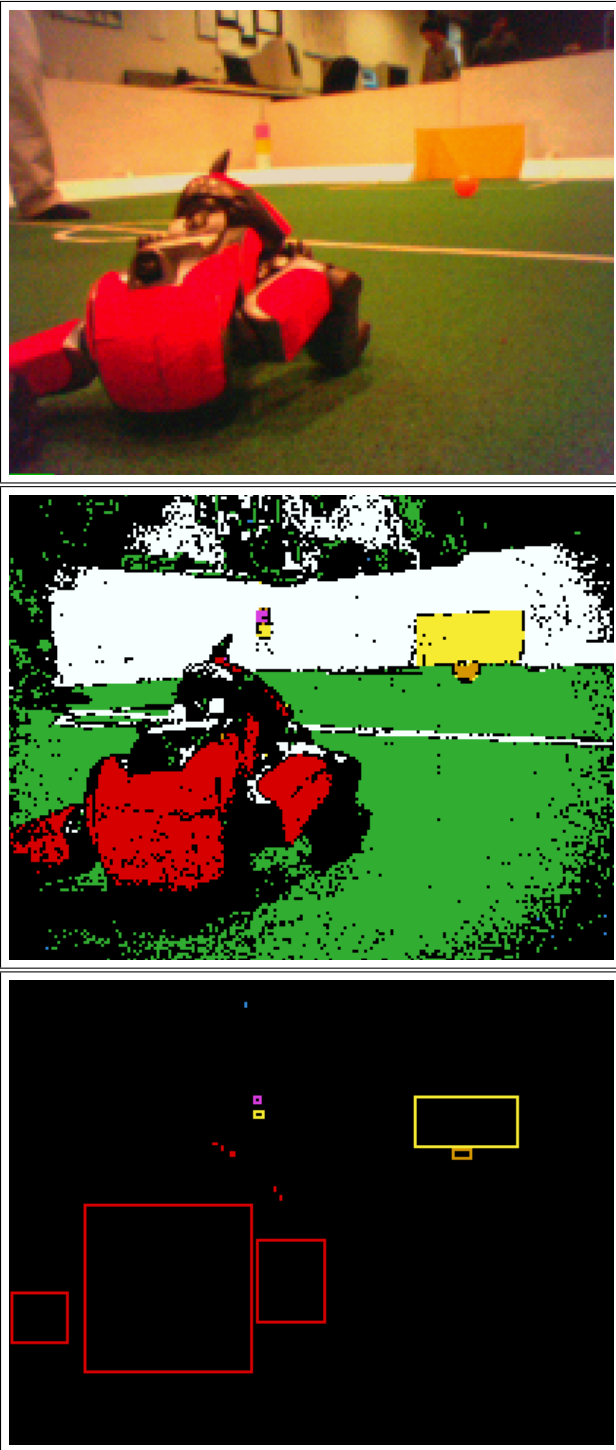
Figure 1: The top figure is the original, unprocessed image obtained from the robot's camera. The middle figure is the same image after colour classification has been performed. The lowest figure shows coloured blobs that have been formed based on the colour classified image.
